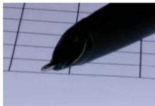
Figure 2. Two pens in one: the pen barrel contains a laser scanner along with a ball point pen.
